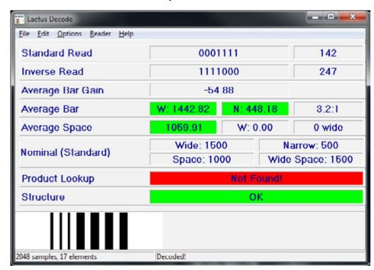
The **Laetus Decode** window provides the binary pattern data followed by the value of the data, and shows this in both directions. All the measurements are expressed in  $\mu$ m (thousandths of a millimetre), and the entries are coloured green or red depending on whether they are in specification. An image of the symbol that has been read is also shown in the window.
