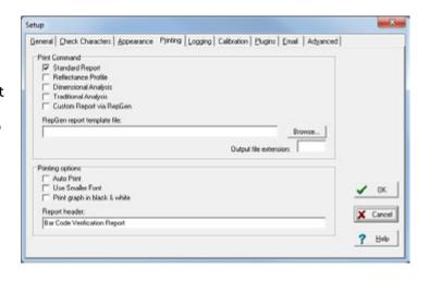
Tick **Print graph in black & white** if you are using a monochrome (black and white) printer, otherwise a scan reflectance profile will only show the outline and not the detail. Also, the standard printed report can be personalised if required using the **Report header**
