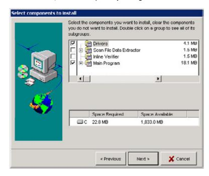
The Scan File Data Extractor enables you to summarise and record all the verifications made in a standalone database. It uses the data from the Axicon scan files (those with a .scn extension) to create a complete record of all the files that have been saved, either automatically or manually. More information about this is available via the website www.axicon.com.
