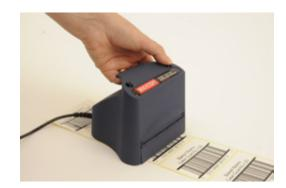
The Axicon 7000 series is being placed flat onto the label with the barcode in the field of view. The 7000 series verifier cannot be used for symbols wider than 200mm, and this dimension includes the quiet zones.
